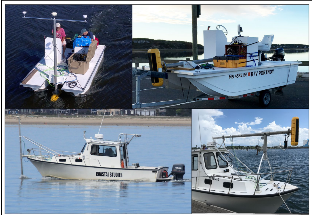
Figure 5. Top: The R/V Portnoy, a custom-built pontoon. An Edgetech 6205 phase measuring sidescan sonar is custom mounted at the bow on both vessels. Bottom: The R/V Marindin.
