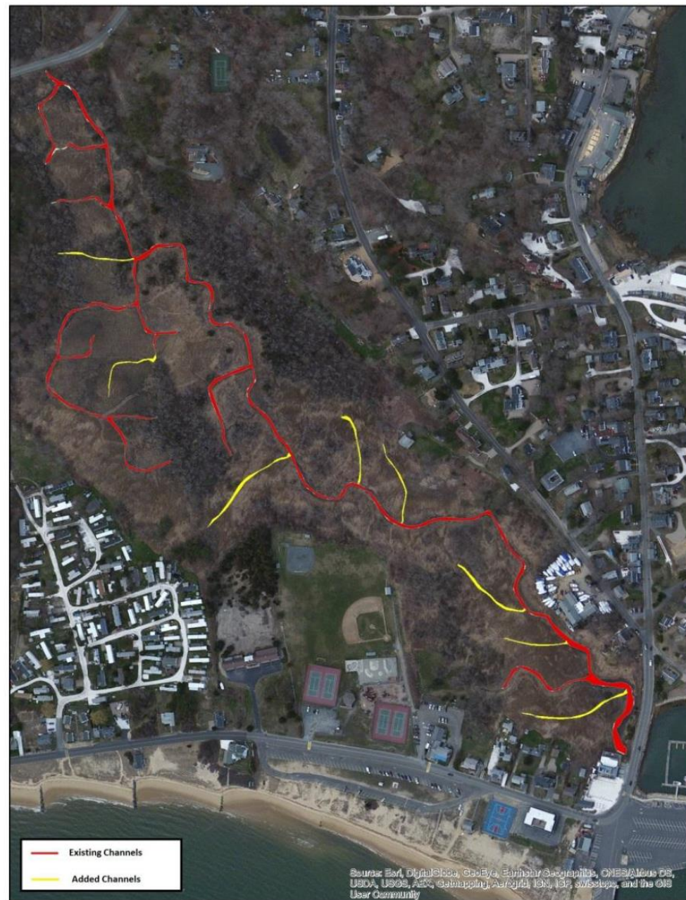
Figure 12. Schematic showing channel lowering (red) and added channels (yellow) for improved drainage.
