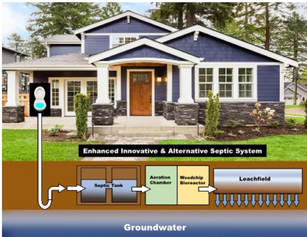
Figure 9 - Enhanced I&A Septic System
