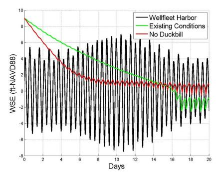
Figure 29. Water surface elevation in Mayo Creek after significant flooding comparing the duckbill removed alternative and existing conditions.
