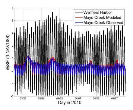
Figure 15. Water surface elevation time series for validation period.
