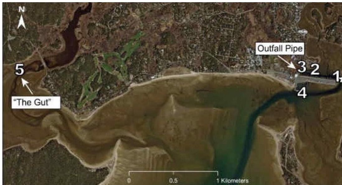
Figure 3. Sediment sample sites from the 2020 Center for Coastal Studies report. According to Table 3 in that report, the median surficial sizes are 39.0, 14.2, 659.5, 24.4, and 542.5 microns, respectively, at sites 1 through 5.
