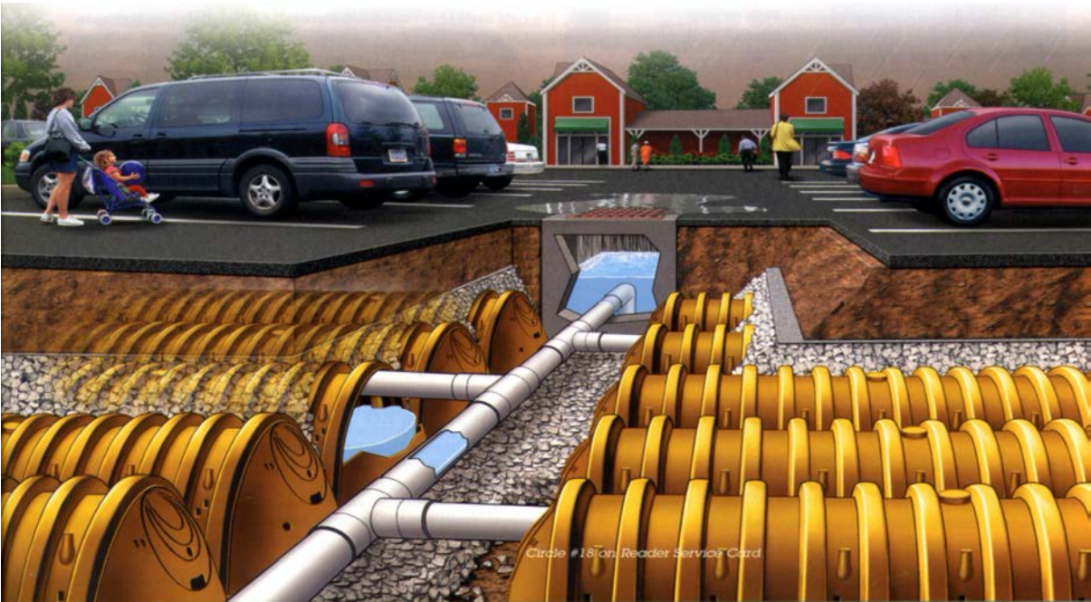
Figure 24 – Stormwater Infiltration with Subsurface Chambers
