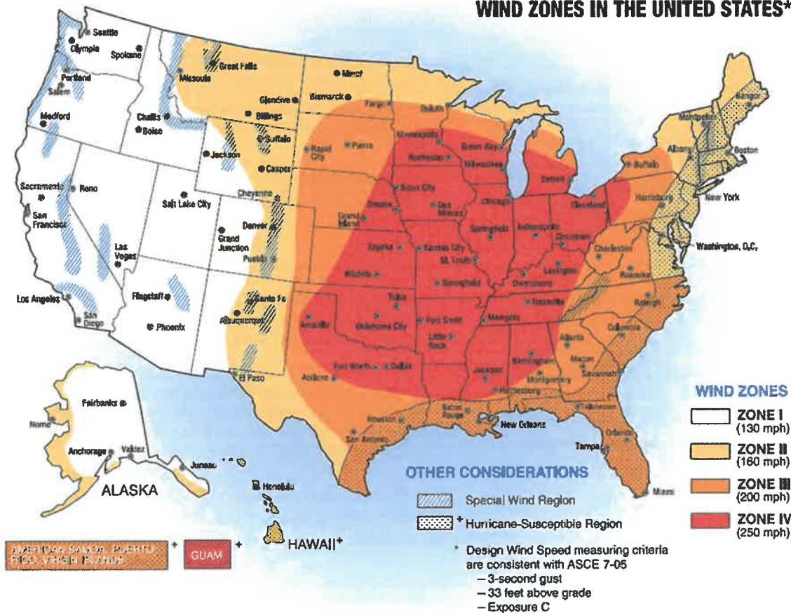
Figure 2.14 | Map of frequency and strength of windstorms in the United States. Planning area is highlighted with a red circle. Map is from the 2013 Massachusetts State Hazard Plan.
