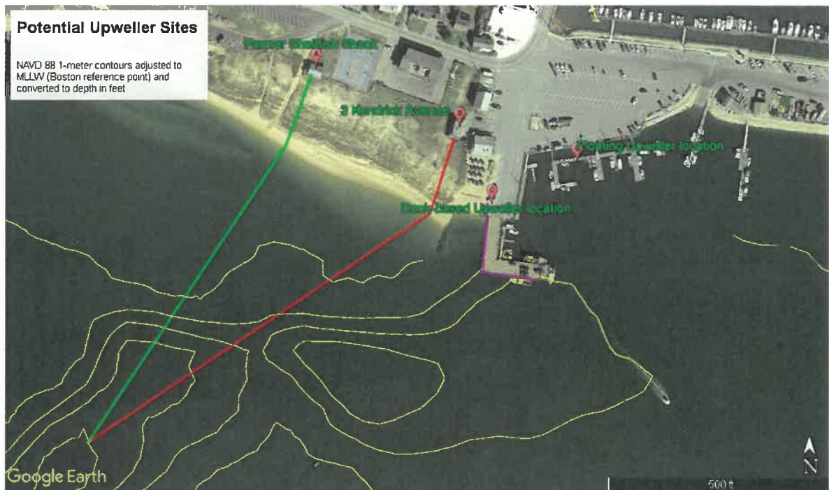
Figure 6. Proposed pathways for the installation of the intake lines for each of the three proposed land-based upweller systems. The respective paths are coded as red for 3 Kendrick Avenue, green for the Shellfish Shack and magenta for the dock-based system.
