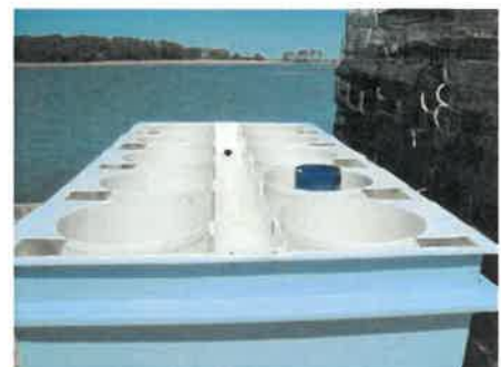
Figure 3. A typical land-based upweller configuration (Barren Island Oyster Company).
