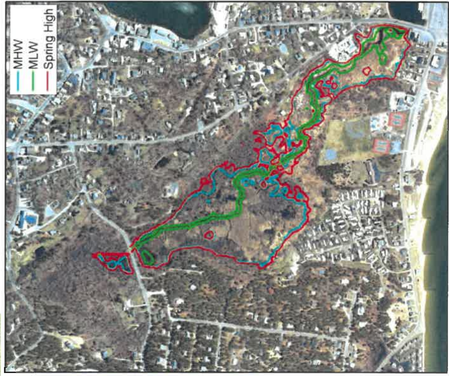
Figure 6. Aerial view of Mayo Creek showing the extent of mean high water (MHW), mean low water (MLW) and spring high tide under a scenario that maximizes salt-marsh restoration without flooding existing infrastructure (Woods Hole Group 2016).
