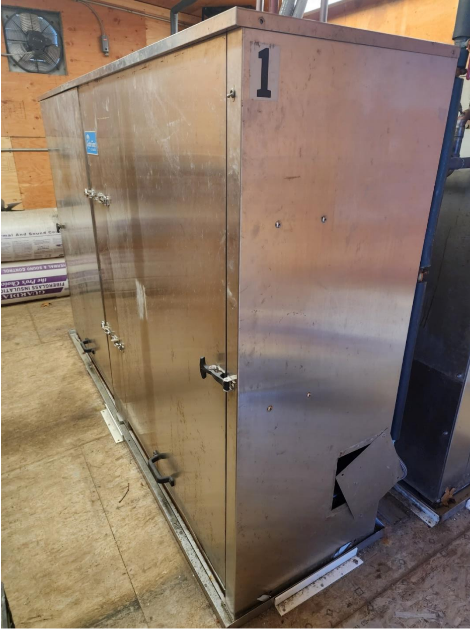
Figure 7 Close up of ice maker - 4 ton
