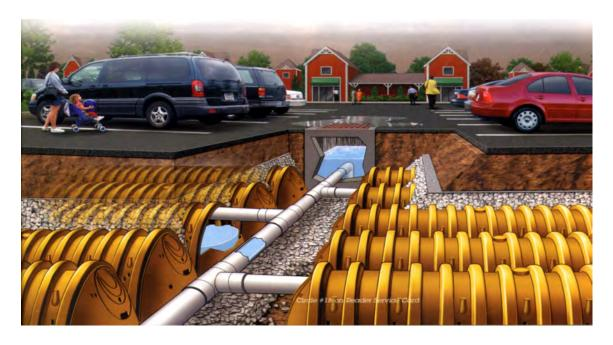
Figure 24 – Stormwater Infiltration with Subsurface Chambers
