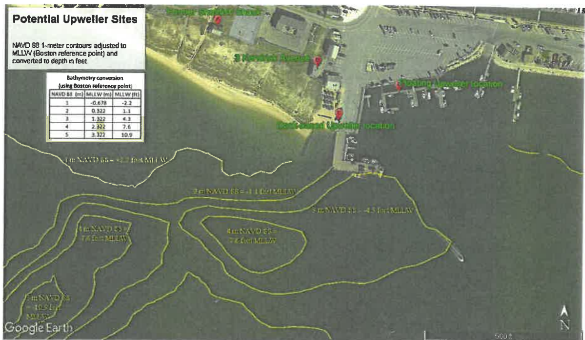
Figure 2. The four locations under consideration for installation of an upweller system in Wellfleet with bathymetry contours adjusted to the MLLW datum (defined in the body of this report) (M. Borrelli, unpublished data).
