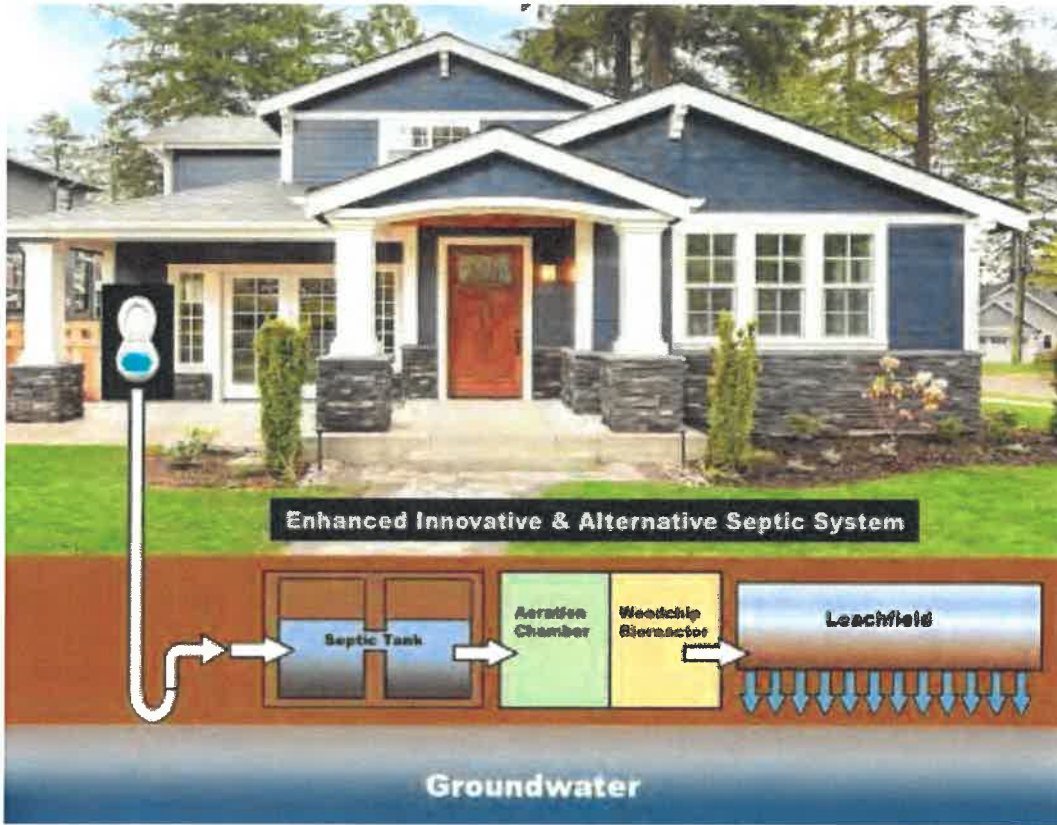
Figure 9 - Enhanced I&A Septic System
