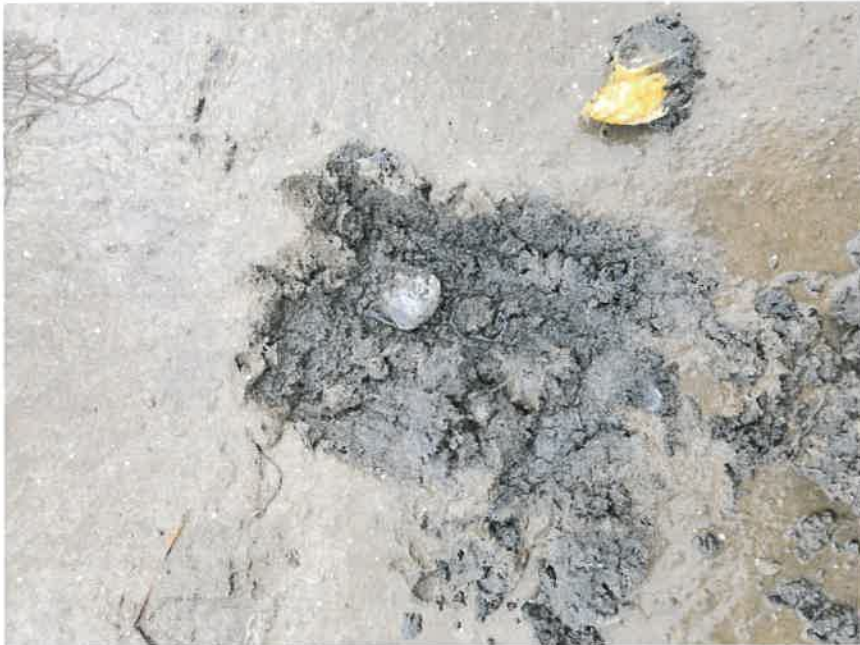
Figure 4: Blackfish Creek typical sediment composed of med / fine sand and some silt.
