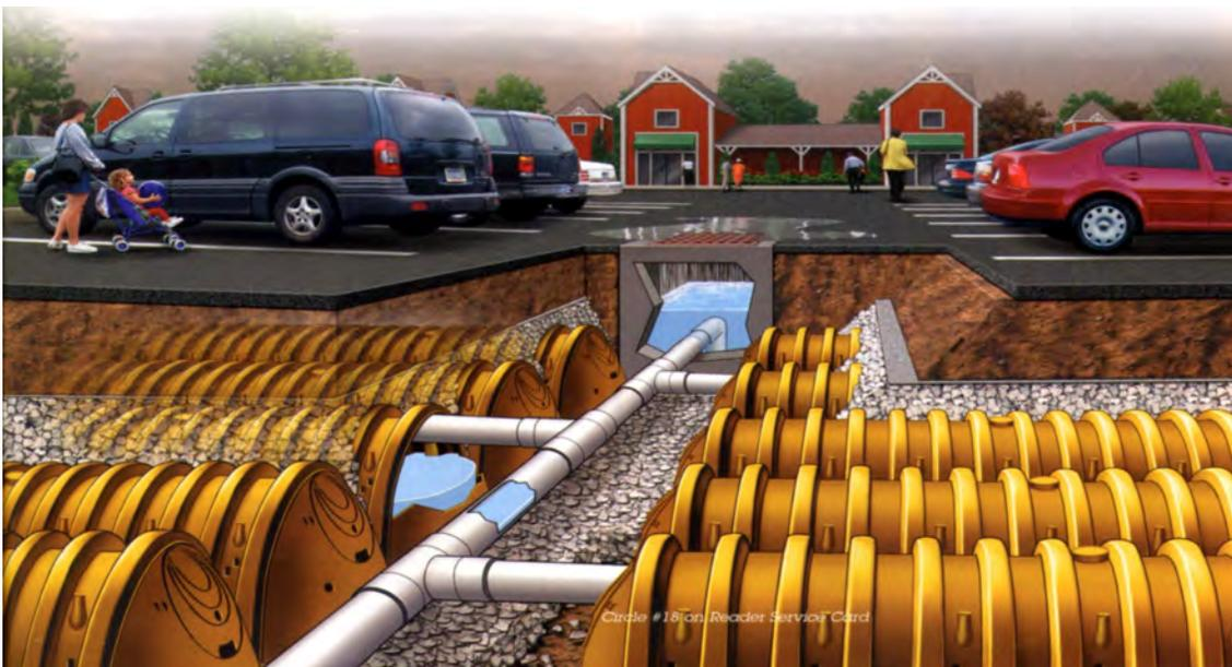
Figure 24 – Stormwater Infiltration with Subsurface Chambers
