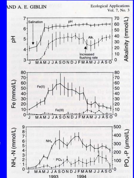
When seawater was added experimentally to Herring River acid sulfate soils for 22 months, pH recovered in 2-3 months, ferrous iron increased and then declined, and ammonium-nitrogen increased in sediment pore water. Cordgrass planted in these microcosm grew very well.
