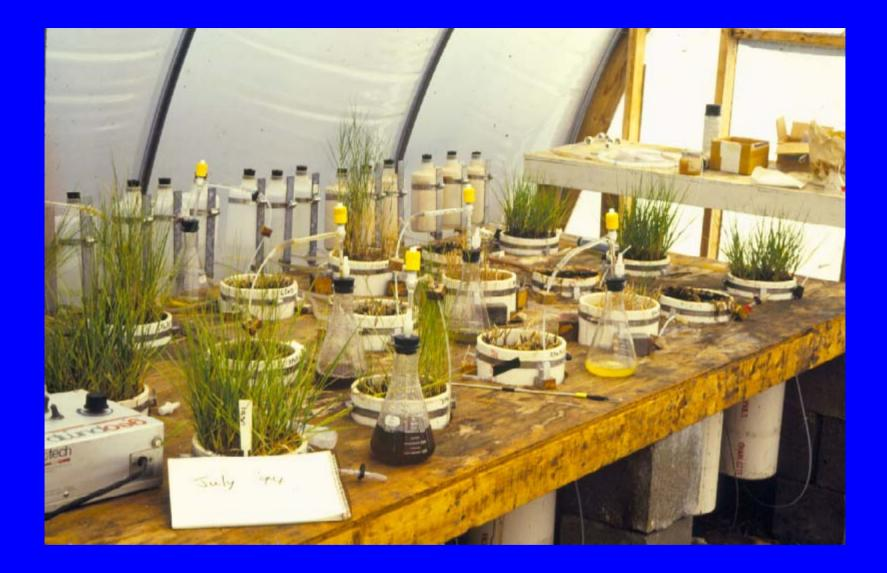
In greenhouse experiments, adding seawater to Herring River's acidified soil eliminated the acidity, and thereby eliminated aluminum toxicity, within two months. Salt marsh grasses grew vigorously in the re-salinated peat.
