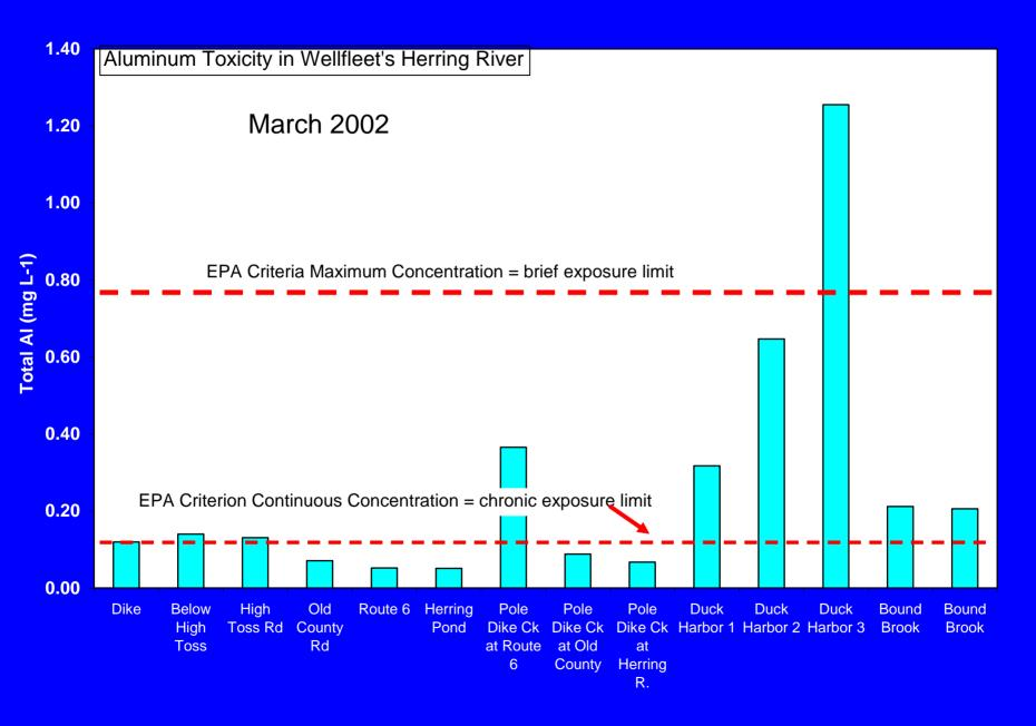
Low pH and high aluminum in Herring River stress and kill fish by damaging gill surfaces, affecting gaseous and ion exchange, and skin, causing lesions.
