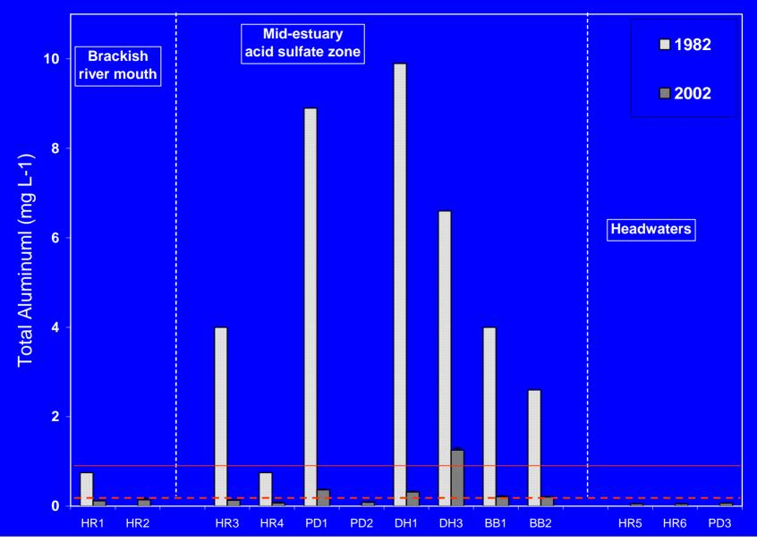
Toxic aluminum in surface water in 1982 and 2002. Conditions have improved, probably due to the elimination of routine stream channelization; however, concentrations still reach EPA's chronic exposure limit (dashed red line) in several streams, and the brief exposure limit (solid red line) in Duck Harbor.
