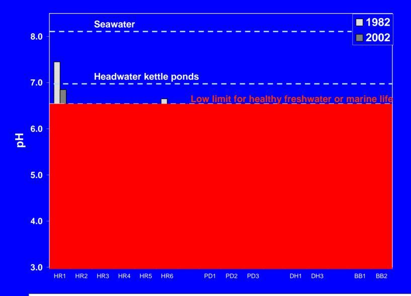
Surface water pH in 1982 and 2002. Most surface waters in the diked Herring River have pH below the EPA limit for healthy aquatic life. There has been some improvement since 1982, probably due to the elimination of regular stream channelization, which exposed stored sulfide minerals to oxidation and acid release.
