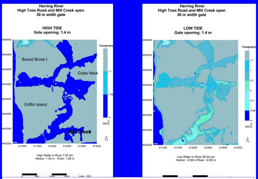
Effects of tidal restoration on tide heights and flushing. Figures show the extent of tidal flooding at high and low tide with the wide-culvert option in the Herring River Dike. This shows an average harbor tide, with 30-meter wide gate open 1.4 m. Note how the system fills at high tide and drains almost completely at low tide, providing both good peat saturation and excellent surface water flushing, i.e. simulating a natural marsh.
